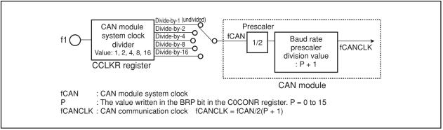
Figure 18.15 Block Diagram of CAN Module System Clock Generating Circuit
